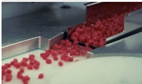
Sample Transfer between Vibrator & Turn-Table
