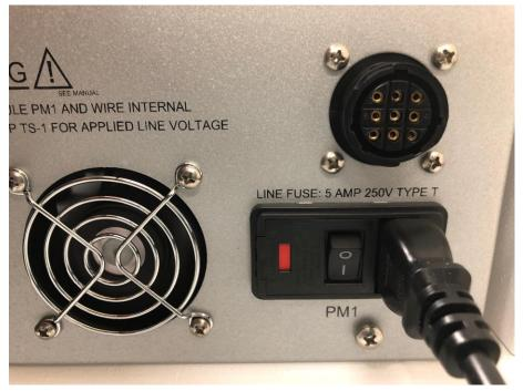
If your system is the HMJ Full Automation package, you will also need to flip the switch found on the right face of the instrument.
